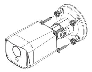
Screw the mounting bracket to the wall or ceiling by using screws(4) and bushings(4) provided with the camera. Adjust the camera angle by bending the stand. After fully assembling the joint screws, unscrew it 2 ~
