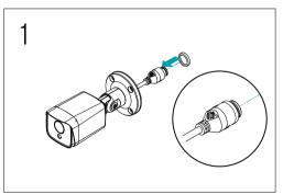
Insert a round rubber ring (silicone rubber) into the RJ45 jack.
