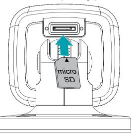
Push the SD memory card until it disengages from the slot, and then pull it out.
