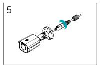
5 Push the waterproof cap body and cap into the RJ45 jack and rotate it.
