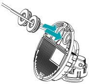
5 Use the screws, anchor provided with the camera to secure the bottom cover on a wall or a ceiling.
