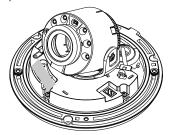
6 Use the screws, anchor provided with the camera to secure the install body on a wall or a ceiling.
