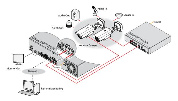
DirectlP $^{\text{TM}}$  NVR makes it easy to use cameras without extra network configurations. Each camera can be controlled via the DirectlP $^{\text{TM}}$  NVR setup menu, without any PC. For detailed camera settings, please see the camera setting pages of DirectlP $^{\text{TM}}$  NVR manual.
