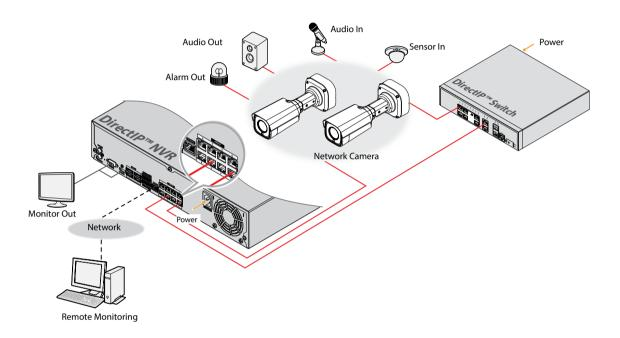
DirectIP™ NVR makes it easy to use cameras without extra network configurations.
