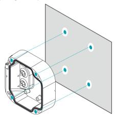
2 After wiring the cable, assemble the body to the bracket hinge. Tighten the screws of the hinge.
