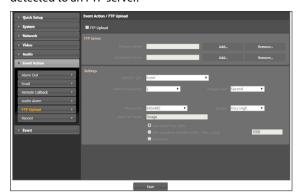
• FTP Server: Click Add to register a new FTP server. Click Remove to remove a registered FTP server. When an event is detected, a .jpg image of the event detected image is uploaded to the Primary Server. If the upload to the Primary Server fails, the file will be uploaded to the Secondary Server. Upload to the Secondary Server will continue to be attempted until successful. Fill out the fields below and click Test to test the FTP server connection settings. Once the test is complete, click OK.
