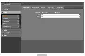
• **Mirroring**: Select Horizontal Reverse or Vertical Reverse to flip the image horizontally or vertically.
