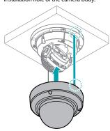
Fasten the screws for the dome cover clockwise using the allen wrench.
