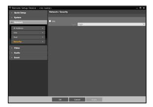
SSL: Select this option to enable SSL (Secure Sockets Layer). Enabling this option applies SSL protocol protection on data transmitted out. However, programs and systems that do not support SSL will not be able to connect to the video encoder. If this option has been changed, Remote Setup will terminate after applying the current settings.
