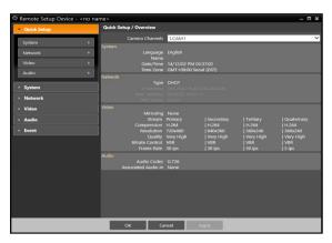
Quick Setup allows you to set up **System**, **Network**, **Video**, **Audio**, and other basic settings needed for video encoder use.
