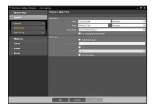
Date/Time: Change the video encoder's date/time settings and display formats and configure the time zone and daylight saving time settings. Click Apply to apply the changes right away.
