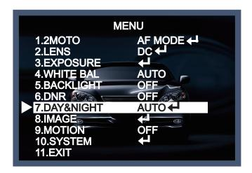
◆ AUTO : Automatically, It shifts into the color mode in the bright environment and the B/W mode in the low light condition. It can adjust the delay time, starting brightness and end brightness according to the ambient conditions by pressing the Set button.
