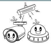
Severe lighting change or flicker can cause the camera to work improperly.
