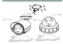
If it gets wet, wipe dry immediately. Liquids can contain minerals that corrode the electronic components.
