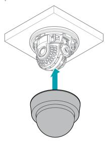
Press the area where the triangular mark meets the side hole cable to assemble the dome cover.
