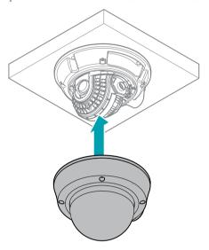
2 Fasten the screws for the dome cover clockwise using the allen wrench provided with the camera.
