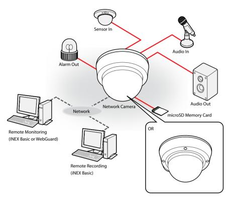
Control the camera over the network from software installed on a computer. Ideal for using the camera over the network from a remote location.
