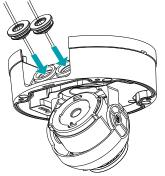
4 Attach the enclosed desiccant in the bottom to prevent moisture.
