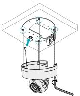
6 Connect external devices, the network cable, and the power adapter.
