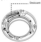
5 Connect the safety wire with the bracket. Fasten the screws for the bottom cover clockwise using the allen wrench provided with the camera.
