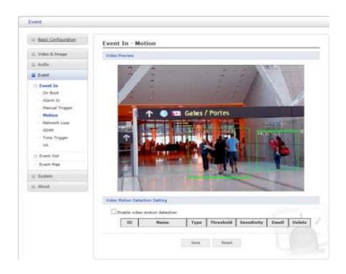
This option makes use of the motion detection function with 16 programmable areas, 8 **Include** and **Exclude** zones each.
