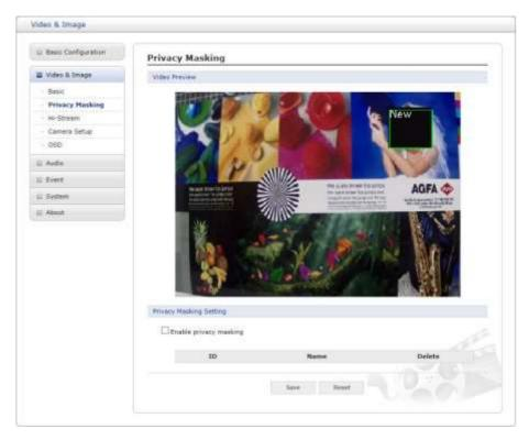
The privacy masking function allows you to mask parts of the video image to be transmitted. You can set up to eight privacy masks.
