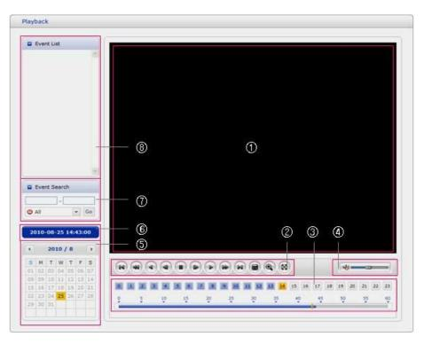
The Playback window contains a list of recordings made to the memory card. It shows each recording's start time, length, the event type used to start the recording, calendar and time slice bar indicates if the recording is existed or not.
