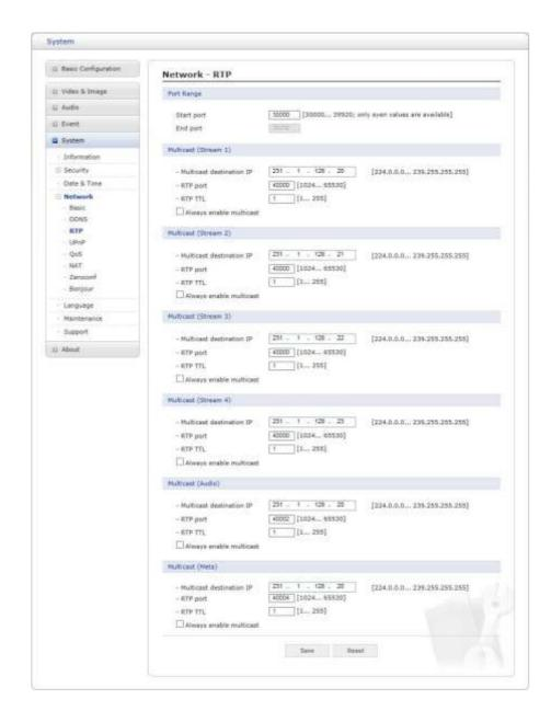
Create a setting for sending and receiving an audio or video on a real-time basis. These settings are the IP address, port number, and Time-To-Live value (TTL) to use for the media stream(s) in multicast H.264 format. Only certain IP addresses and port numbers should be used for multicast streams.
