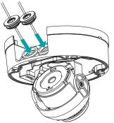
4 Connect the safety wire with the bracket. Fasten the screws for the bottom cover clockwise using the allen wrench provided with the camera.
