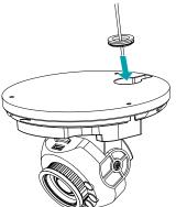
3 Use the screws, anchor provided with the camera to secure the body on a wall or a ceiling.
