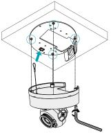
5 Connect external devices, the network cable, and the power adapter.
