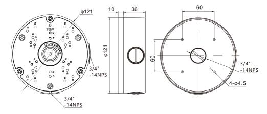
There are three pipe thread interface in the junction box, one of which needs to be used, so our company provides two plugs.
