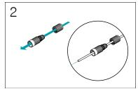
Insert the network cable into the waterproof cap, rubber bushing, and waterproof cap body in order.
