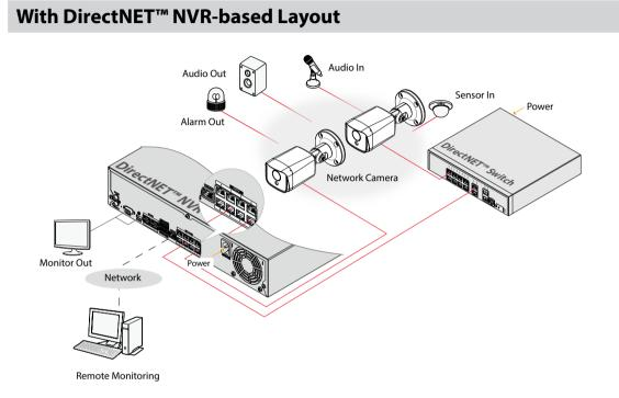
DirectNET<sup>™</sup> NVR makes it easy to use cameras without extra network configurations. Each camera can be controlled via the DirectNET<sup>™</sup> NVR setup menu, without any PC. For detailed camera settings, please see the camera setting pages of DirectNET<sup>™</sup> NVR manual.
