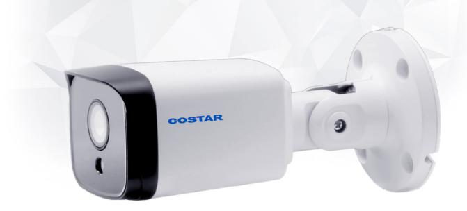
The CBI5D4IW DirectNET Bullet camera provides high quality video at 5 megapixel resolution. The infrared LEDs provide illumination for clear image quality at night. The advanced H.265 codec allows for smaller recording file sizes and lower transmission bandwidth on your network.
