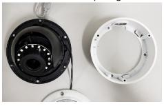
5. Using a Phillips screwdriver remove the three (3) bolts that that secure the multi-purpose mounting plate from the junction box.
