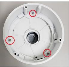
12. Remove the twist tie from the camera main cable. Make the video and power connections. Feed the excess cable into the junction box.
