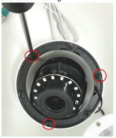
4. Remove the camera from the back housing by twisting the back housing counterclockwise and pulling down.
