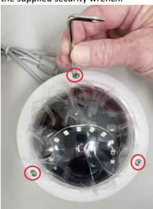
3. Use a Phillips screwdriver to remove the three (3) bolts that secure the Camera to the back housing.
