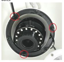
14. Use the supplied security wrench to tighten the three (3) security bolts on the camera dome.
