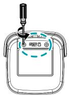
2 Insert a SD memory card into the SD memory card slot with the 'micro SD' print facing upward.
