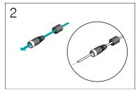
2 Insert the network cable into the waterproof cap, rubber bushing, and waterproof cap body in order.
