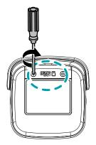
Make sure that the cover is joined properly when screwing it; otherwise, the IP67 level is not guaranteed.
