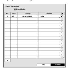
Highlighting Schedule On and pressing the 🗗 button toggles On and Off. When set to On, you can select the day, time range and interval that you want the DVR to run self-diagnostics on the recorder. The Interval can be selectable from 1 min. to 7 days or Never. Highlight the + and press the 🗗 button to add a schedule item. The 🗙 box allows you to delete a check recording schedule.
