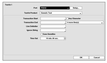
Highlight the box beside Port, and press the 🗗 button. Select from None, RS232, RS485, USB-Serial (1~8) and LAN (1~16).
