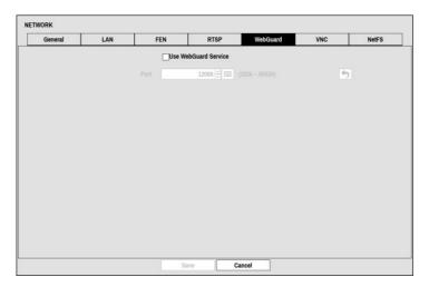
Figure 33: Network - WebGuard setup screen.
