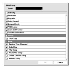
Highlighting the Authority box and pressing the 🗗 button will toggle between all authority levels being turned On and Off. Highlighting the individual authority level boxes and pressing the 🗗 button will toggle between that authority level being turned On and Off. The authority levels that can be turned On and Off are:
