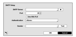
Highlight the box beside SMTP Server and press the button. A virtual keyboard appears that you can use to enter the IP address or domain name of the SMTP server. Highlighting allows you to select your SMTP server from a list of registered SMTP servers.
