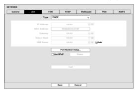
Selecting DHCP from the Type and highlighting Save button reads the current IP address of the DVR configured by DHCP (Dynamic Host Configuration Protocol) network.
