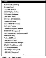
and press the button. A list of PTZ devices appears. Select your camera from the list and press the 🗗 button. You will need to connect the camera to the RS232 or RS485 connector on the back of the DVR following the camera manufacturer's instructions.
