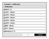
You can toggle the entire list On and Off by highlighting Notification and pressing the without button. You can toggle the individual items On and Off by highlighting that item and pressing the without button. Highlight OK and press the without to accept your changes.
