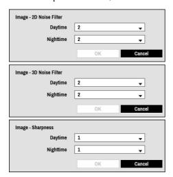
Each function can be applied between 1 (Weak)  $\sim$  5 (Strong) in strength, according to Daytime/Nighttime.
