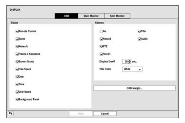
Figure 40: Display - OSD setup screen.
