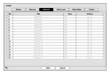
Figure 17: Event - Alarm-In setup screen.
