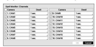
You can define which cameras display sequentially on the Spot Monitor when in the single-screen display format. Highlighting the box under the Camera and pressing the button toggles between On and Off.
