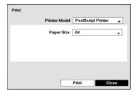
Highlight the box beside Printer Model and press the ← button. Selecting PostScript Printer will print images on a PostScript<sup>™</sup> printer connected to the DVR. Selecting File Printer will save the current image as a PDF file on an external USB hard disk drive or flash drive or a NetFS site.
